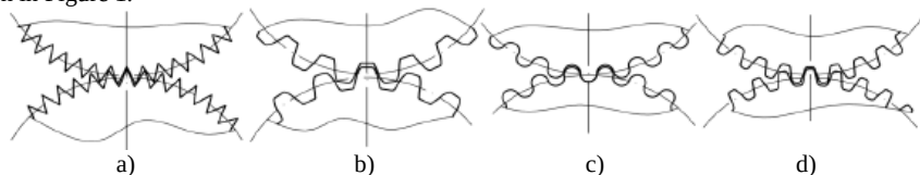
Fig. 1. Types of gear engagements of decorticator rollers:
